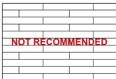
Brick bond installation 50% (NOT RECOMMENDABLE)
